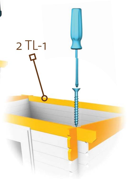
INSTALL THE **ROOF** PURLINS AND **ATTACH** THEM WITH SCREWS.
