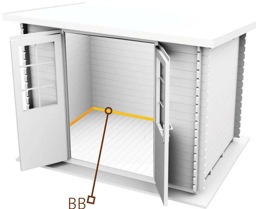
DRILL THROUGH THE WALL, HOLE MUST BE AT THE BOTTOM OF THE OVAL, ATTACH WITH BOLT.
