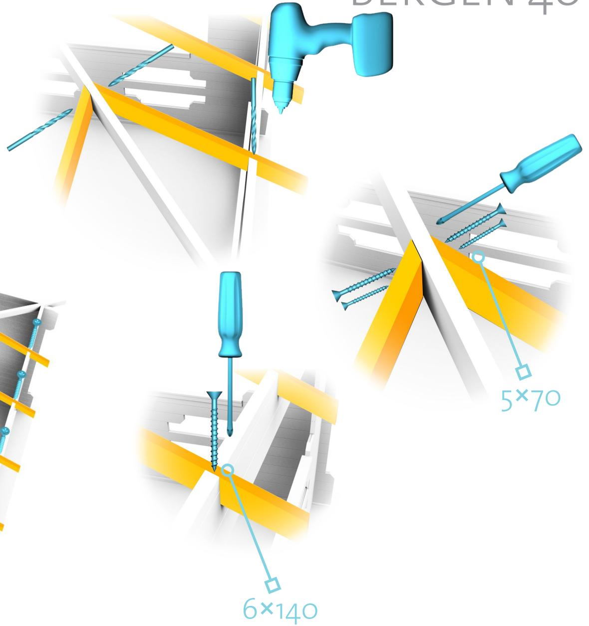
PLACE THE FIRST ROOFBOARD FLUSH WITH THE END OF THE PURLINS AND ATTACH WITH SCREWS
