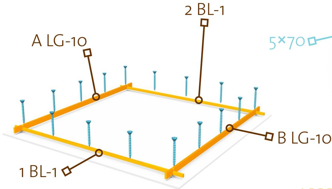
THE WALL LOGS WILL HANG OVER THE FOUNDATION BEAMS BY APPROXIMATELY 5MM. THIS OVERHANG IS DESIGNED AS A RAIN DRIP. 3%
