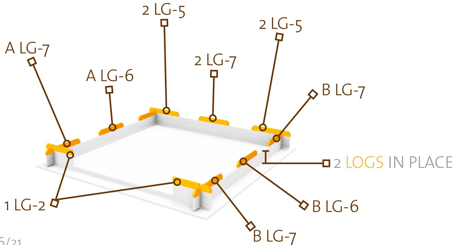
AFTER PLACING 3-4 ROWS OF WALL LOGS, TAP EACH WALL LOG IN PLACE USING A HAMMER AND THE HITBLOCK PROVIDED, TO TIGHTEN THE LOGS.
