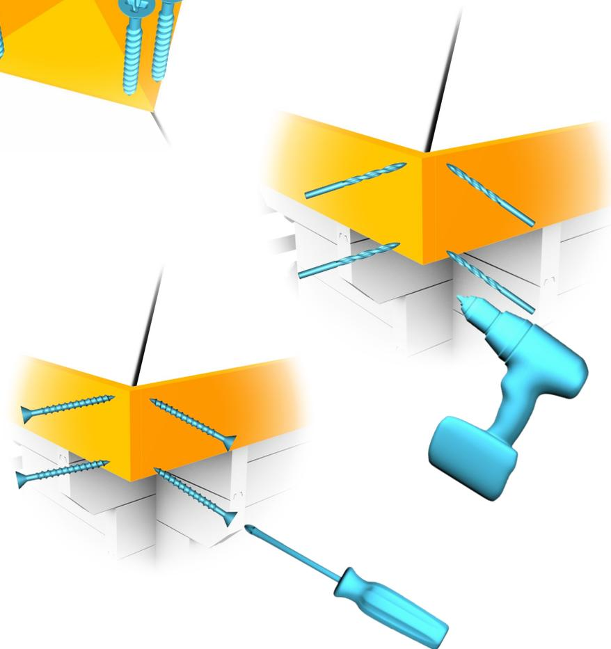
WINDBOARD CONNECTS BOTTOM LOG WITH THE TOP LOG. SAW THE WINDBOARD INTO THE RIGHT LENGTH. FOR THE TOP BOLT, DRILL 8MM HOLE THROUGH THE WINDBOARD.
