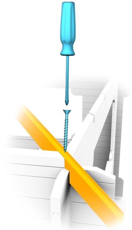
INSTALL THE **ROOF** PURLINS (RFB) AND ATTACH THEM WITH SCREWS.
