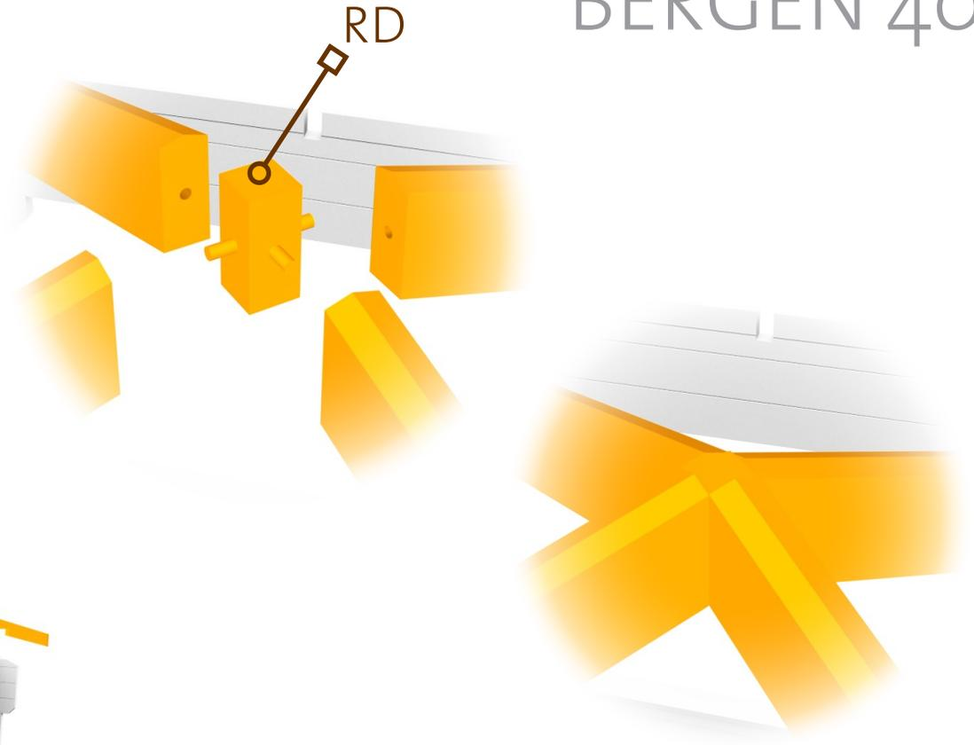
INSTALL THE **ROOF** PURLINS AND ATTACH THEM WITH SCREWS.
