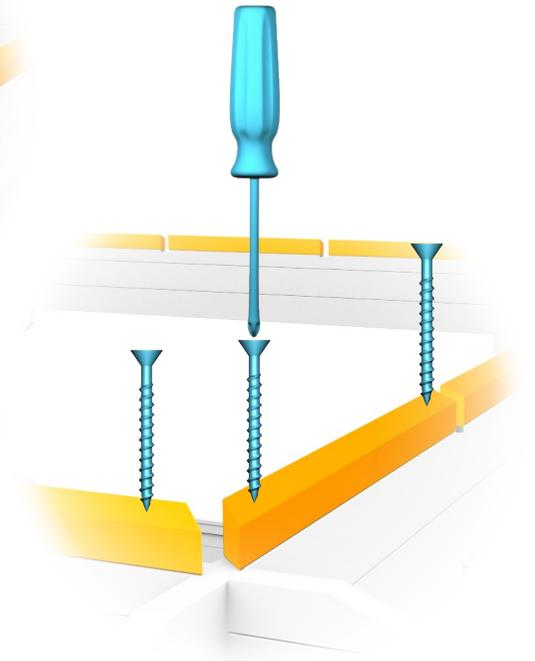
CONNECT THE ROOF PURLINS (RFR) WITH RD BEFORE INSTALLING THEM ON TOP OF THE CORNERS.
