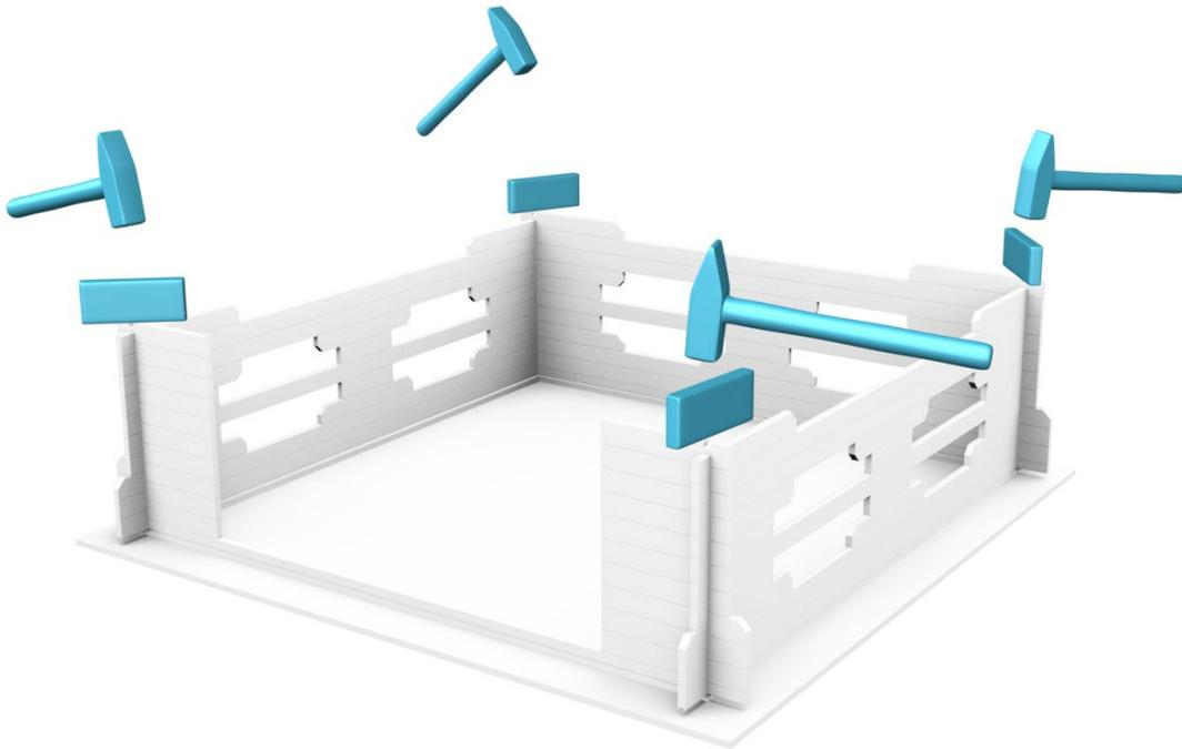
ATTACH **HANDRAILS** INTO WALL LOGS WITH SCREWS.
