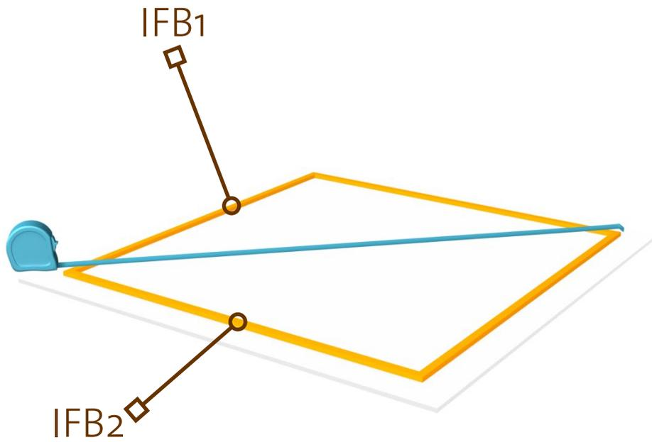
MAKE SURE THAT THE FOUNDATION IS INSTALLED ON A LEVEL SURFACE. CHECKING ALL DIRECTIONS, INCLUDING CORNER TO CORNER. 1%
