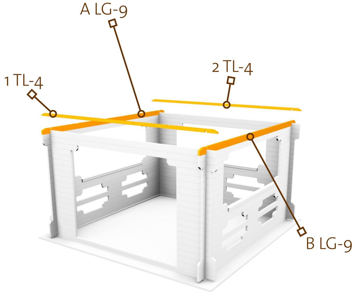
ATTACH TOP LOGS INTO WALL LOGS WITH SCREWS.
